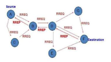
Fig. 2 Example of a AODV Routing Protocol
